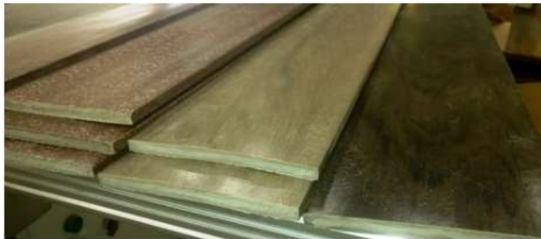
Panel core layer: Epoxy-glass fibre FRP-waste / recycled HDPE-plastic (70/30%)
